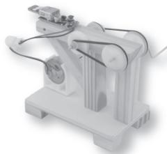
07 - Cut the foam tape into the same size as the bottom of the booster plate and stick the booster plate to the position shown in the figure. Then put on the rubber band to connect the small pulley and double pulley. Finally, put on the other two belts and install the USB light.
