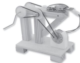
08 - Connect the booster plate and motor with the wires.
