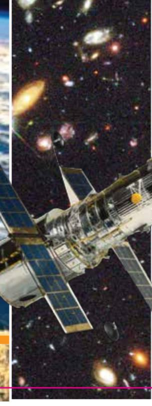
**9** The Hubble Space Telescope, 13.3 m/43.5 ft long—the length of a large school bus, was sent into orbit on April 25, 1990. The telescope is one of the most significant advances in astronomy since Galileo's telescope in 1609. Although Hubble may not travel directly to the stars, planets, or galaxies, it flies around Earth at 17,000 mph and captures amazing pictures of them. Since 1990, Hubble has made more than 1.2 million observations.
