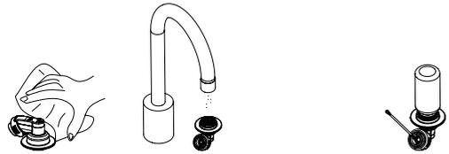
1. When using essential oils with different aroma, it is recommended to wipe atomizing module with a clean cotton cloth or rinse the inside of the atomizing module with water.
