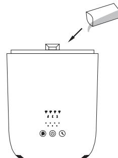
**3.** Pour water into the water tank up to the maximum level indicated (2L). Never put water into air outlet which will cause unit malfunction.
