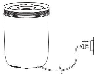
**6.** Plug the adaptor into the appropriate outlet.
